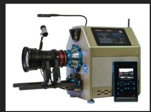
users to check the lens itself for offset back focus, optical distortions or zoom-smoothness.
